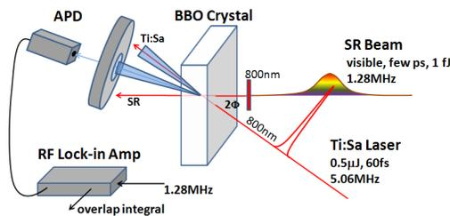
Figure 2: Mixing with am 800nm Ta:Sa laser.
