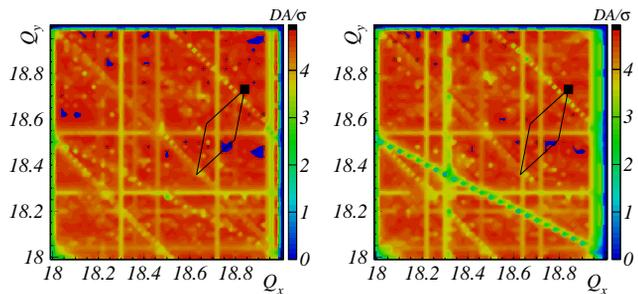
Figure 4: DA scan obtained by removing the 3rd order components in dipoles (left); Right) DA scan obtained by correcting  $Q_x + 2Q_y = 56, 3Q_x = 56$ .
