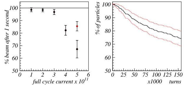
Figure 3: Left) Summary of the beam survival at the end of the cycle. Right) Beam survival of the first injected bunch with  $0.625 \times 10^{11}$  ions for dipoles with all multipoles reduced by a factor of 2.
