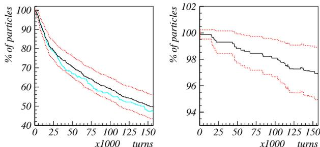
Figure 5: Survival of the first bunch beam for the case  $0.625 \times 10^{11}$  ions, without resonance compensation (left), and with resonance compensation (right).
