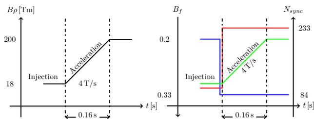
Figure 6: Schematic of the acceleration ramp (left); Change of bunching factor and of the synchrotron tune (right).
