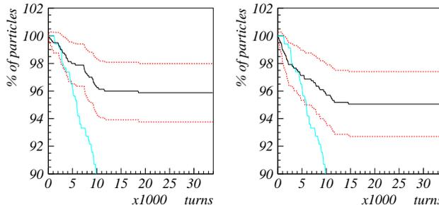
Figure 7: Beam loss during the  $4T/s$  ramp without including eddy current (left). On the right picture the systematic eddy current is included. In blue the beam survival at injection plateau (for comparison).
