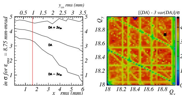
Figure 1: DA vs. COD (left); Statistical results of DA scan (right), the black marker shows the working point.
