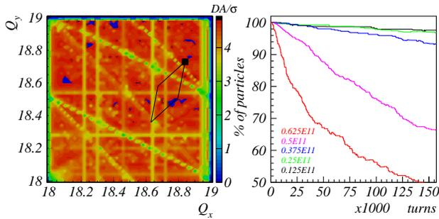
Figure 2: DA scan for the reference error seed and the expected tune-spread (left). First bunch survival evolution for several beam intensities (right).
