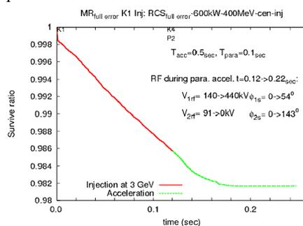
Figure 7. Survival ratio of power upgrade scenario with new power supply.
