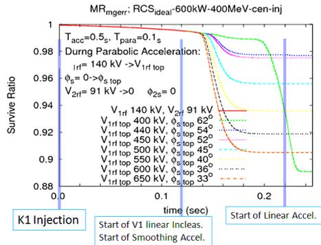
Figure 5. 2.5D simulation results of survival ratio of a proton bunch injected at 1<sup>st</sup> injection timing with changing top voltage of main RF.
