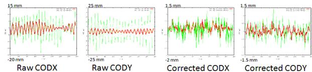
Figure 2. Raw COD and COD corrected by steerers. Red lines are with August 2010 magnetic alignment, and Green lines are with Jun 2011 magnetic alignment. Horizontal axis is MR longitudinal position.
