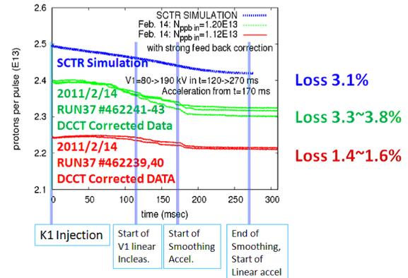
Figure 1. Beam survival time structure in MR FX operation. Blue line is 2.5D simulation (with SCTR code) result. Green lines are experimental results corresponding MR 145 kW FX operation. Red lines are experimental results corresponding MR 133 kW FX operation. Same color lines mean different shots under the same condition.
