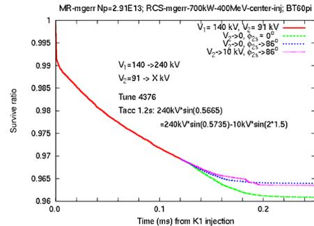
Figure 8. Survival ratio of power upgrade scenario with current power supply. Green line is for  $V2=91$  kV to 0 during smoothing and  $\phi_{2s}=0$ , blue line is for  $V2=91$  kV to 0 and  $\phi_{2s}=0$  to 86 degree during smoothing, and purple line is for  $V2=91$  kV to 10 kV and  $\phi_{2s}=0$  to 86 degree during smoothing.
