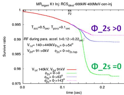
Figure 6. Effect of  $\phi_{2s} > 0$  pattern on beam survival ratio. Conditions are the same as  $V1\_top=440$  kV case in Fig. 5 except for  $\phi_{2s}$  pattern. Green line is for  $\phi_{2s} = 0$ , and it is the same as blue line in Fig. 5.
