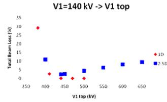
Figure 4. Beam loss ratio depending on top voltage of main RF, V1\_top. Red marks are 1D simulation results. Blue marks are 2.5D simulation results including transverse space charge effect.
