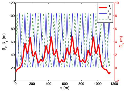
Figure 2: Nominal optics (Q26) of the SPS (1/6 of the circumference). The phase advance per FODO cell is close to  $\pi/2$ , resulting in a total phase advance of  $\mu_x \approx 4 \cdot 2\pi$  per arc and thus 4 big oscillations of the dispersion function.
