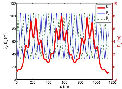
Figure 4: New optics with low  $\gamma_t$  (Q20). The phase advance per cell is reduced to  $3/8\pi$  resulting in a phase advance of  $3 \cdot 2\pi$  per arc with 3 big dispersion oscillations in the arcs and dispersion suppression in the straight sections.
