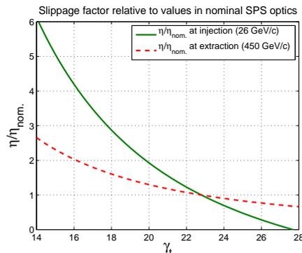
Figure 1: Slippage factor  $\eta$  relative to the value of the nominal optics (nominal  $\gamma_t = 22.8$ ) as a function of  $\gamma_t$ . At injection  $\gamma = 27.7$  and at extraction  $\gamma = 480$ .
