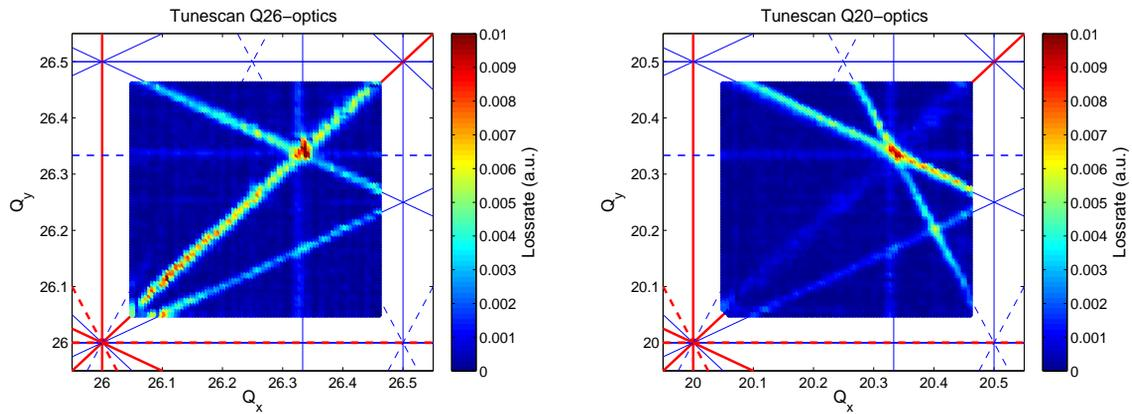
Figure 5: Experimental tune scans in the SPS with the nominal (Q26) optics (left) and the low  $\gamma_t$  (Q20) optics (right). The color-code indicates the loss rate during a dynamic scan of the fractional tunes. The underlying tune diagram shows resonances up to third order, with systematic resonances in red and non-systematic in blue. Solid lines correspond to normal and dashed lines to skew resonances.
