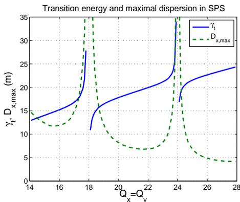
Figure 3:  $\gamma_t$  and maximal dispersion around the ring as function of horizontal tune ( $Q_y$  set equal to  $Q_x$ ). For  $Q_x$  close to multiples of the machine super periodicity 6, resonant oscillations of the dispersion function are induced which result in the asymptotic behavior of  $\gamma_t$ .
