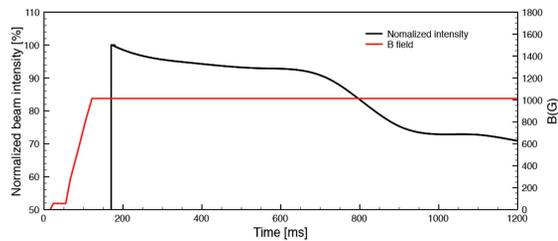
Figure 1: Magnetic cycle used for the 1.4 GeV measurements with the signal from the beam current transformer normalized to the injected intensity.
