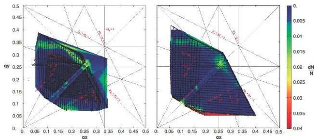
Figure 4: Tune scan results at 2 GeV, for two different settings of non-linearities introduced by the PFW. The resonance  $2Q_h+2Q_v=1$  appears to be different.
