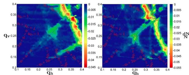
Figure 3: Tune scan results at 1.4 GeV, for a bunched beam (left), and a debunched one (right). The color scale indicates the derivative of the BCT signal, i.e., the red lines indicate the larger losses.
