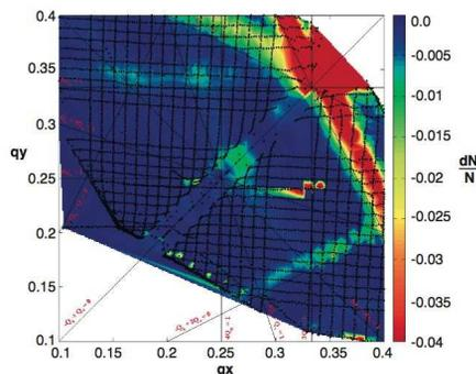
Figure 2: Tune diagram resulting from the loss measurement at 2 GeV. The color scale indicates the derivative of the BCT signal, i.e., the red lines indicate the larger losses. The measurement points are indicated by the black dots.
