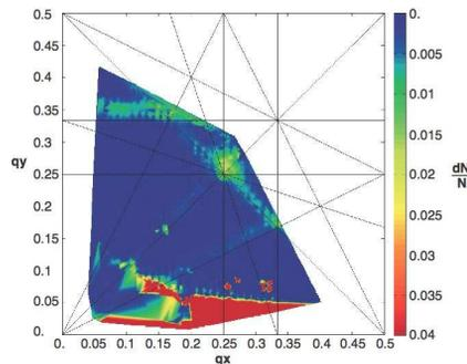
Figure 5: Tune scan results at 2 GeV to approach the integer resonance.
