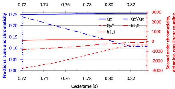
Figure 2: Overview of the time-evolution of the main parameters  $h_{2,0}$ ,  $h_{0,2}$ ,  $h_{1,1}$  together with the horizontal tune and the linear and second order chromaticity during the splitting process.
