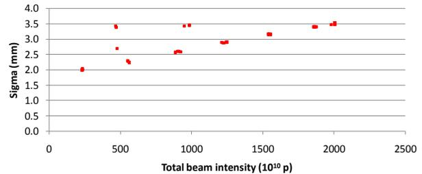
Figure 3: Horizontal beam size before resonance crossing as a function of the total beam intensity. A linear dependence is clearly visible, due to the multi-turn injection process in the PS-Booster. The outliers represent the cases in which the number of bunches has been reduced.
