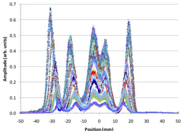
Figure 4: Superposition of the horizontal beam profiles measured after splitting for various beam intensities. The displacement of the four outermost beamlets is visible.
