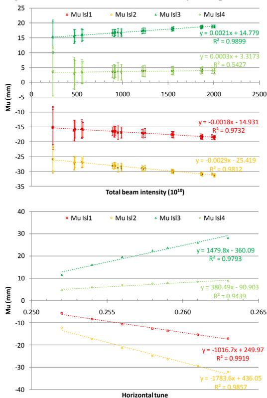
Figure 5: Beamlets position vs. intensity (upper) from the fit of the profiles showed in Fig. 4. Fixed point position vs. horizontal tune (lower) from the numerical PS model.
