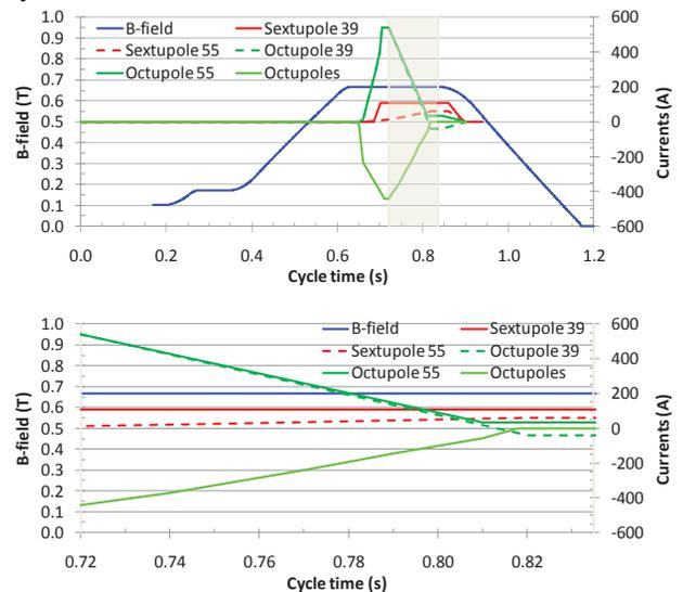
Figure 1: Overview of the MTE gymnastics (upper). The magnetic cycles is shown together with the evolution of the current in the non-linear elements used for generating the stable islands and correcting the non-linear coupling. The shaded area represents the region where the transverse splitting takes place: the zoom of this region is shown in the lower plot. The numbers after the elements indicate the straight section in which they are installed.
