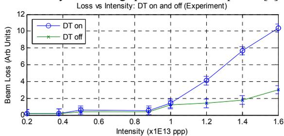
Figure 1: Measured loss vs intensity, driving term on, off.
