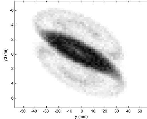
Figure 6: Density plot in single particle phase space ( $y, y'$ ) showing expected half integer structure (ORBIT).
