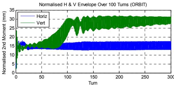
Figure 4: Evolution of horizontal and vertical envelopes over 300 turns, parameters as Figure 3.
