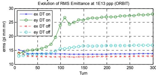
Figure 3: Evolution of  $\epsilon_{rms,x}$ ,  $\epsilon_{rms,y}$  over 299 turns, with driving term on and off, and intensity  $1.0 \times 10^{13}$  ppp.
