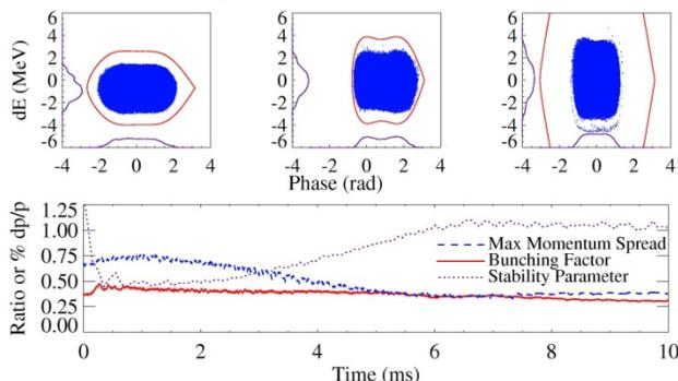
Figure 2: Phase space at 0, 5, 10 ms for  $8 \times 10^{13}$  ppp and evolution of bunching factor, stability parameter (equation 2) and maximum  $dp/p$  for scheme one.
