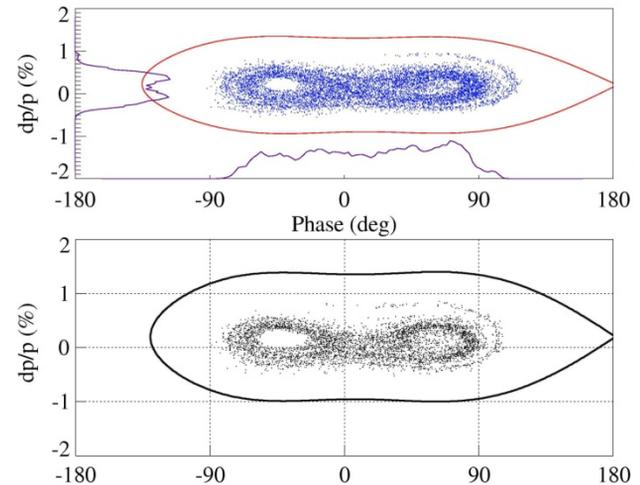
Figure 4: Phase space at the end of J-PARC injection simulated using the ISIS code (top) and the J-PARC code (bottom, [8]).
