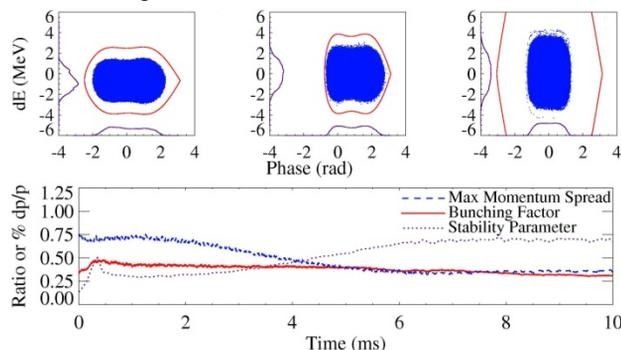
Figure 3: Phase space at 0, 5, 10 ms for  $8 \times 10^{13}$  ppp and evolution of bunching factor, stability parameter (equation 2) and maximum  $dp/p$  for scheme two.
