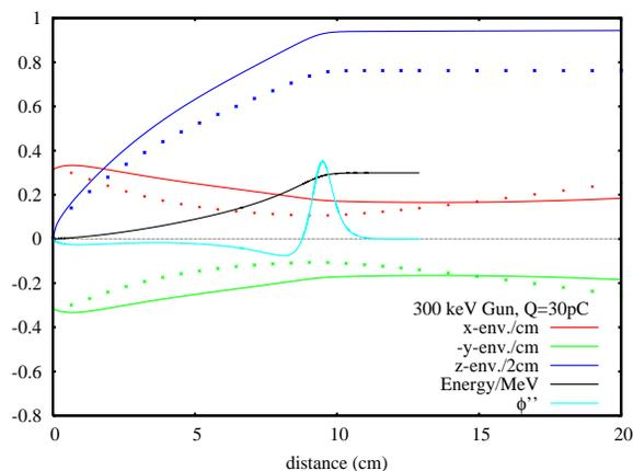
Figure 1: Beam envelopes calculated from a cathode,  $Q = 30$  pC bunches accelerated to 300 keV in a distance of 9.5 cm. The case without space charge is shown dotted for comparison.
