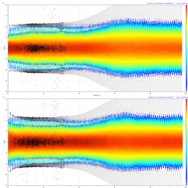
Figure 3: Particles density plot on transverse plane X along the RFQ, for the constant B case, upper plot, and the low B case, lower plot.
