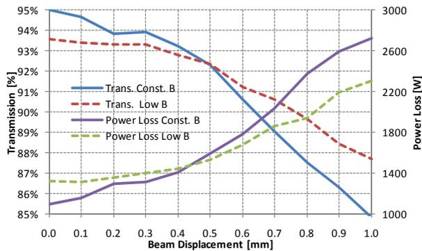
Figure 6: Transmission and power loss as function of beam displacement for the Constant B and the low B RFQ.
