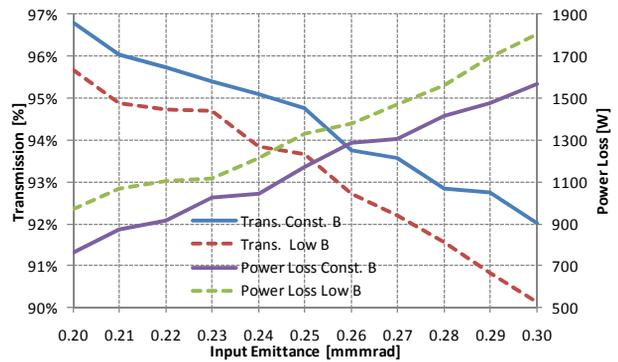
Figure 8: Transmission and power loss as function of the input emittance.
