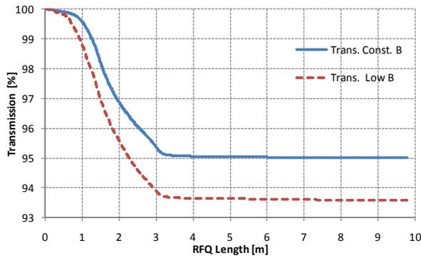
Figure 5: Transmission along the RFQ.
