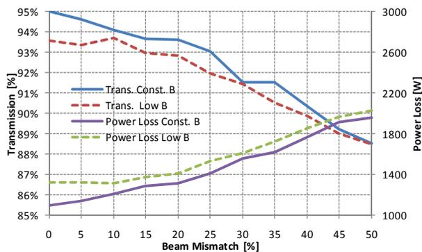
Figure 7: Transmission and power loss as function of the beam mismatch.
