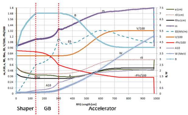
Figure 2: Main parameters evolution along the RFQ.
