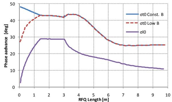
Figure 1: Comparison of phase advance at zero current for the constant B RFQ, and for the low B RFQ.
