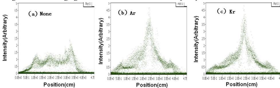
Figure 3: beam profile variation in SCC effect. (a)no extra gas added. (b)Ar as compensation gas, pressure is  $2.9 \times 10^{-3}$  Pa. (c)Kr as compensation gas, pressure is  $2.1 \times 10^{-3}$  Pa.
