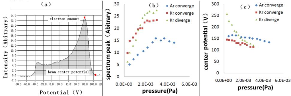
Figure 2: (a)Typical energy spectrum. (b)Energy spectrum peak in different conditions. (c) Beam center potential in different conditions.
