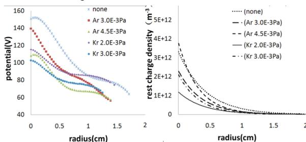
Figure 5: (a) Beam potential distribution, fitted by polynomial. (b) rest charge density distribution, fitted by indicial equation.
