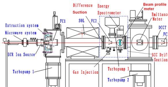
Figure 1: Scheme of the test bench, read calligraphy indicates the facilities specially for the SCC study.
