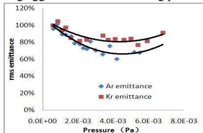
Figure 4: Emittance variation in Kr and Ar compensation. All data is compared with the emittance value without extra gas injection.
