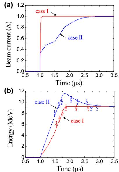
Figure 2: Temporal profile of the beam energy for different beam current shapes: Case I, the square beam pulse; Case II, the modulated beam current. The RF is injected at 1  $\mu$ s with a square pulse. The beam currents shown in (a) are measured values, which are used to obtain the beam energies, shown in (b). For the beam energies in (b), the lines are theoretical values and the dots are experimental values.
