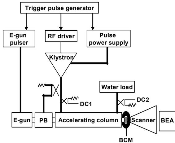
Figure 1: Schematic diagram of the L-band accelerator (left end: RF input coupler, right end: RF output coupler).
