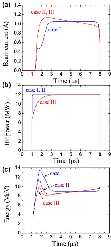
Figure 3: Compensation effect on the beam energies induced by modulation of the beam current and RF power: Case I, before compensation; Case II, beam current modulation; Case III, Case II + RF power modulation. The beam energies in (c) are theoretical values.
