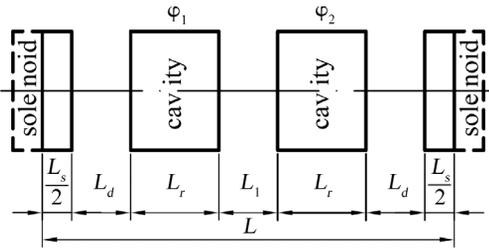
Figure 1: Layout of structure period.
