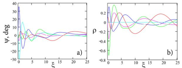
Figure 2: The longitudinal and transverse phase trajectories of the particles during the acceleration.
