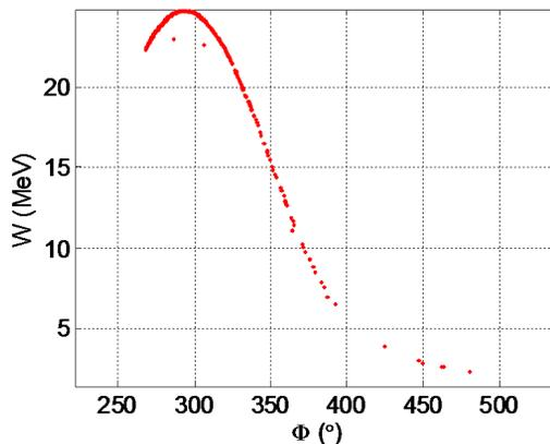
Figure 3: Steady state phase-energy distribution of particles at the exit of the first section.
