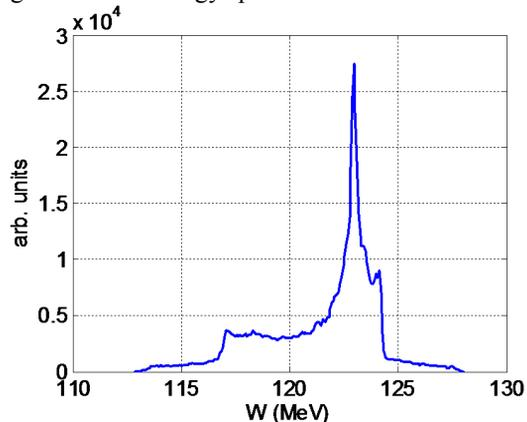
Figure 6: Energy spread on the target for the whole current pulse.
