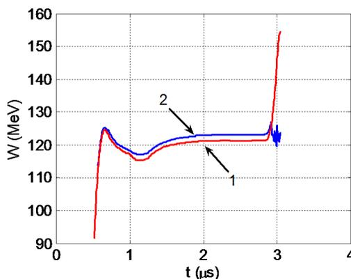
Figure 4: Average beam energy within current pulse at the linac exit (1) and after the bend (2).
