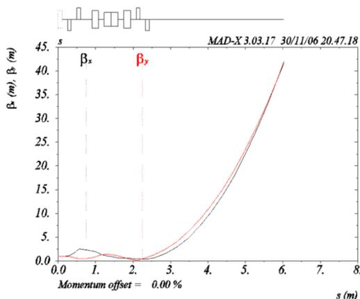
Figure 2: Chicane optic functions.
