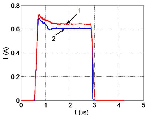
Figure 5: Beam current at the linac exit (1) and after the bend (2).
