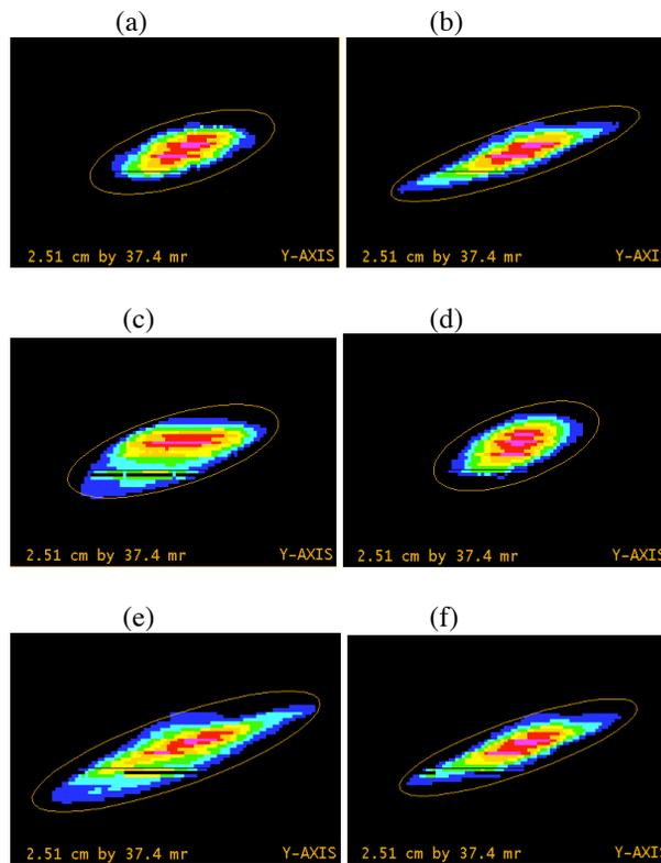
Figure 6. Effect of chopping and bunching on vertical emittance at TDEM1: (a) Chopper Off, Bunchers Off, (b) Chopper Off, Bunchers On, (c) Chopper 36 ns, Bunchers Off, (d) Chopper 290 ns, Bunchers Off, (e) Chopper 36 ns, Bunchers On, (f) Chopper 290 ns, Bunchers On.
