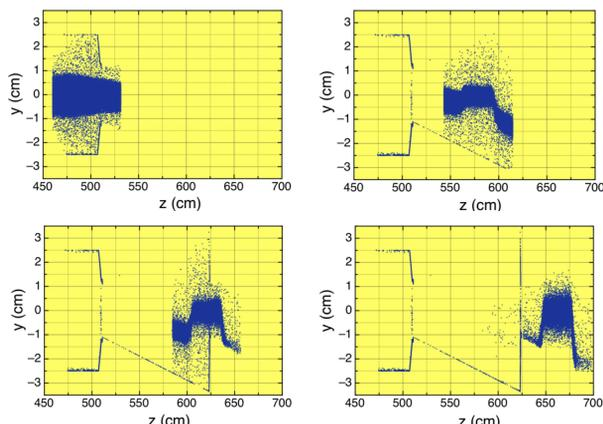
Figure 5. Dynamics of 36 ns beam pulse in chopper.
