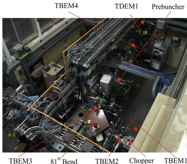
Figure 1. Layout of 750 keV H<sup>-</sup> Low Energy Beam Transport of LANSCE.
