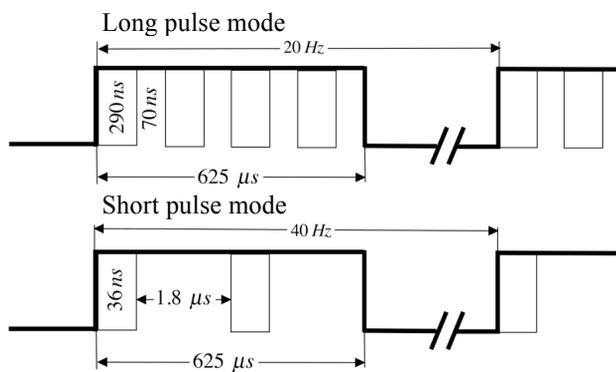
3. Figure 3. Pulse structure of the beam.
