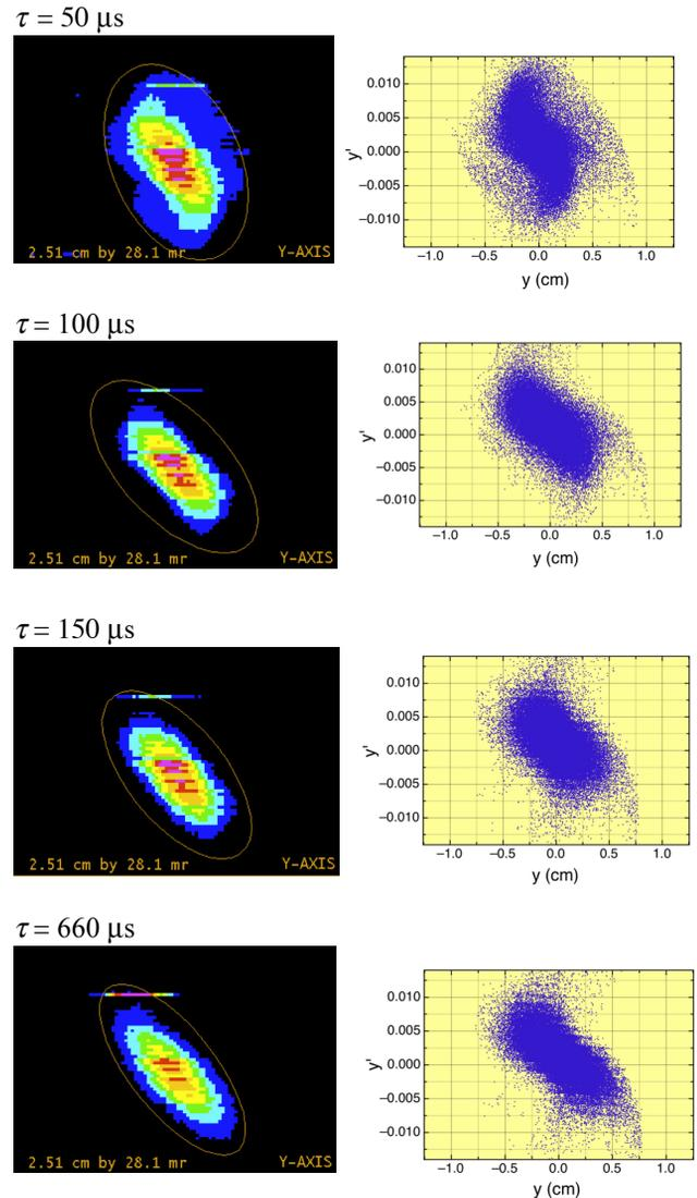
Figure 4. (Left) Measured vertical beam emittance at TBEM3 and (right) BEAMPATH simulations at different values of beam pulse length (simulations performed with current  $I = 15$  mA for  $\tau = 50$ -100  $\mu\text{s}$  and with current  $I = 0$  for  $\tau \geq 150$   $\mu\text{s}$ .)
