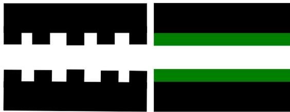
Figure 1: Corrugated waveguide and waveguide with dielectric inner layer.
