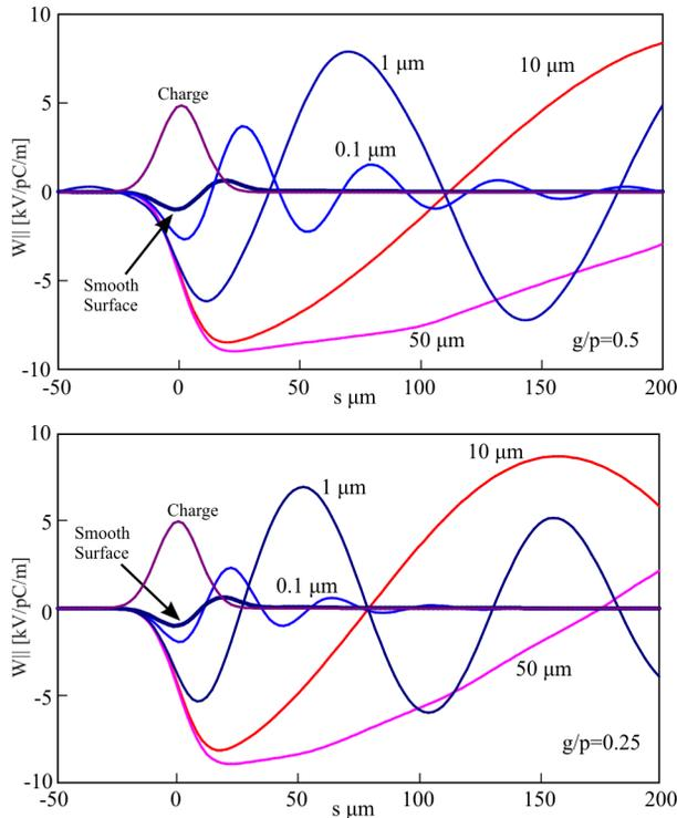
Figure 4: Longitudinal wake potential;  $g/p=0.5$  (top) and  $g/p=0.25$  (bottom)
