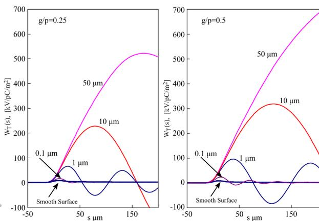
Figure 5: Longitudinal wake potential;  $g/p=0.5$  (left) and  $g/p=0.25$  (right).
