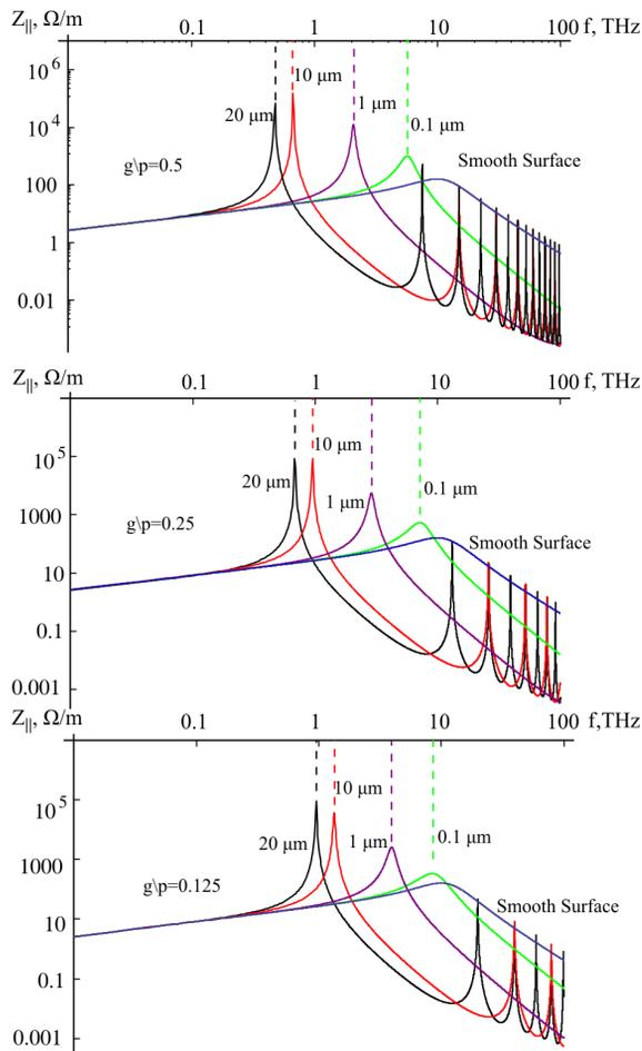
Figure 2: Real part of the longitudinal coupling impedance distributions;  $g/p=0.5$  (top), 0.25 (middle), 0.125 (bottom). Also shown (Smooth Surface) corresponds to the non-corrugated (ideal) case .
