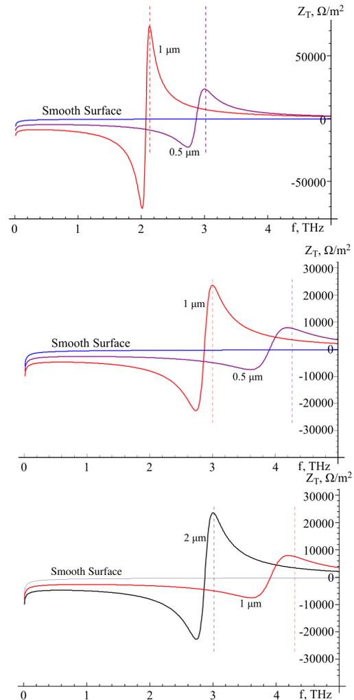
Figure 3: Imaginary part of the transverse coupling impedance distributions;  $g/p=0.5$  (top), 0.25 (middle), 0.125 (bottom). Also shown (Smooth Surface) corresponds to the non-corrugated (ideal) case.
