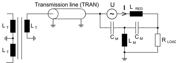
Figure 3: Equivalent electrical circuit used for impedance calculation of the kicker power supply including an additional inductivity  $L_{RED}$  to reduce the coupling impedance.
