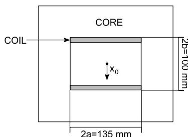
Figure 1: Sketch of the cross-section of a SIS100 window frame kicker magnet.
