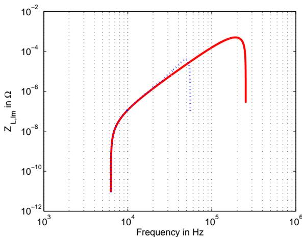
Figure 7: Imaginary part of longitudinal impedance for  $x_0 = 10$  mm. In red without and in blue with the additional inductor.
