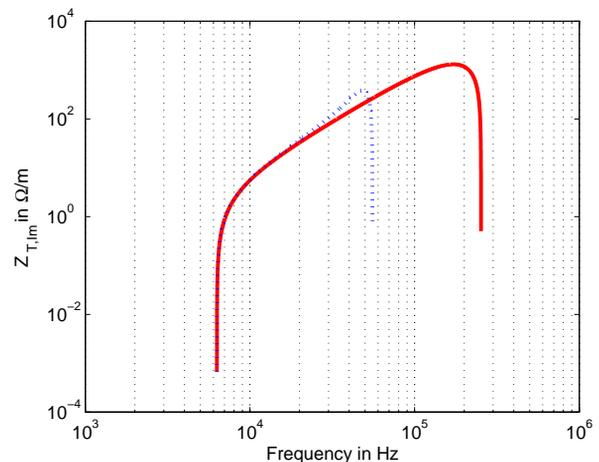
Figure 5: Imaginary part of transverse impedance. In red without the additional inductor and in blue with the additional inductor.
