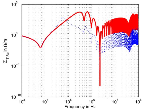
Figure 4: Real part of transverse impedance. In red without the additional inductor and in blue with the additional inductor.
