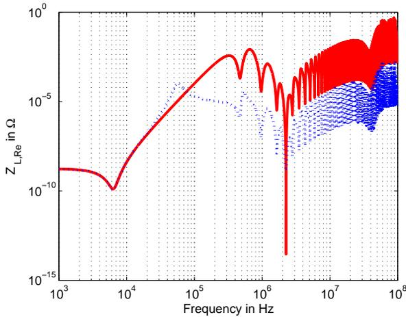
Figure 6: Real part of longitudinal impedance for  $x_0 = 10$  mm. In red without the additional inductor and in blue with the additional inductor.
