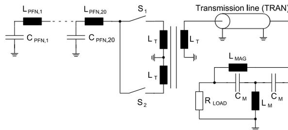
Figure 2: Electrical circuit for the favored set-up of the kicker power supply.
