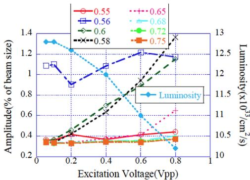
Figure 6: Luminosity degradation and vertical oscillation amplitude for each frequency component excited by white noise.
