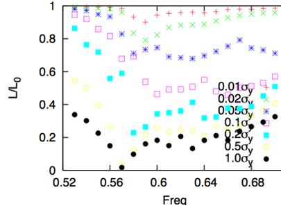
Figure 3: Luminosity response for frequency scan given by the simulation.
