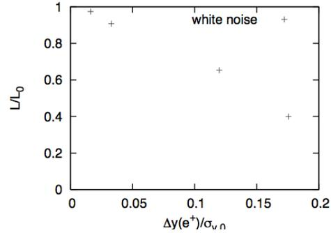
Figure 7: Luminosity degradation and vertical amplitude due to white noise excitation in the simulation.
