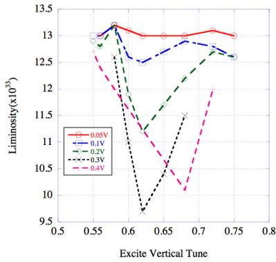
Figure 1: Luminosity response for frequency scan in various voltages. The data 0.60-0.65 at 0.4V is missing because of too strong luminosity loss.
