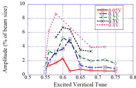
Figure 2: Amplitude of excited oscillation at IP. The data 0.60-0.65 at 0.4V is missing.
