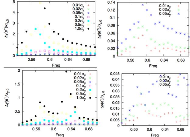
Figure 4: Amplitude of excited oscillation at IP given by the simulation. Top and bottom are positron and electron amplitudes, respectively. Rights are plotted with fine vertical scale. Positron beam is excited by an external sinusoidal noise.
