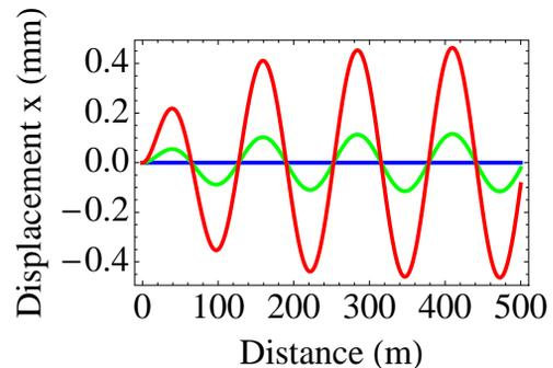
Figure 1: The displacement  $x$  of a point on the bunch as a function of traveling distance. The blue, green and red curve corresponds to the position of head, center and tail particles along the beam respectively.
