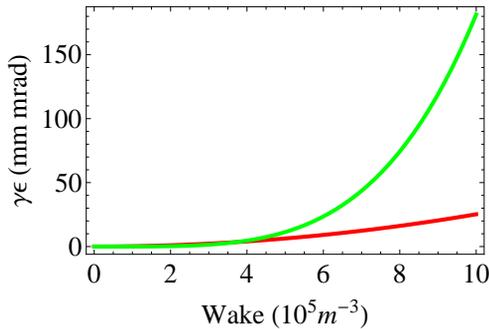
Figure 2: Emittance growth as a function wakefield. The red line and green line corresponds to the 1<sup>st</sup> and 2<sup>nd</sup> order contribution to beam emittance growth respectively.
