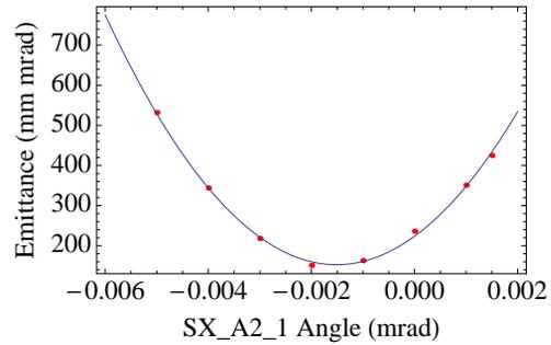
Figure 4: Emittance as a function of kick angle. The red dots are the emittance value of 5 nC beam. The blue line is the parabolic data fitting. The KEKB linac lattice file has been implemented into Elegant, and the components have a random misalignment of 0.5 mm.
