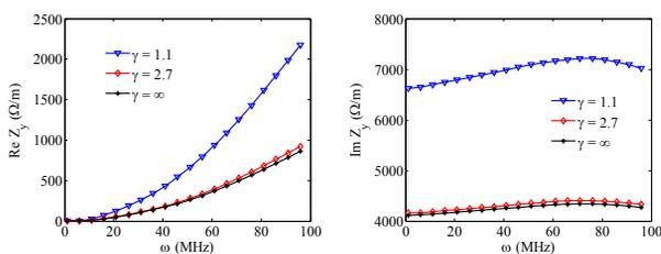
Figure 3: Vertical coupling impedance of a typical kicker of CSNS/RCS. Left and right plots show the real and the imaginary parts, respectively.
