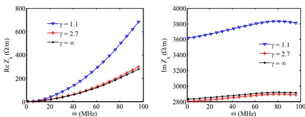
Figure 2: Horizontal coupling impedance of a typical kicker of CSNS/RCS. Left and right plots show the real and the imaginary parts, respectively.
