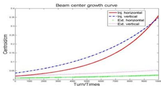
Figure 2: Injection and extraction transverse bunch centre variety versus turn in CSNS/RCS. The red, blue and green, pink lines are injection horizontal, vertical and extracted horizon, verticality plane respectively.
