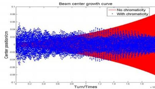
Figure 4: Varied energy resistive wall instability growth curve vs chromaticity in CSNS/RCS. The red curve is transverse growth no chromaticity, the blue curve denotes growth with natural chromaticity.
