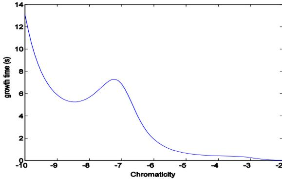
Fig 1: Injection transverse growth time versus chromaticity.
