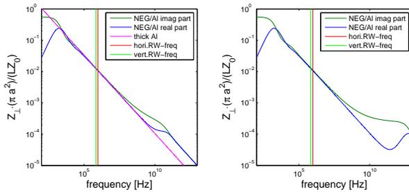
Figure 3: RW-impedance of  $1.5\mu$ -NEG-layer on Al chamber, left resistivity  $\rho = 2.5 \cdot 10^7 \Omega m$ , right  $\rho = 5.5 \cdot 10^4 \Omega m$
