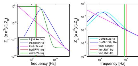
Figure 2: RW impedance of ceramic kicker chamber with  $0.4\mu$  Ti-cover(left), and RW impedance' real part of Cu/Ni-sheet for  $50\mu$  res.  $100\mu$  layer thickness,  $Z_0 = 377\Omega$ .
