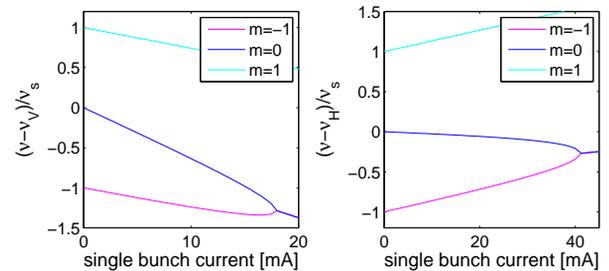
Figure 5: single bunch mode detuning in phase I computed by MOSES, left vertical, right horizontal. The quadrupolar wake field is taken into account.
