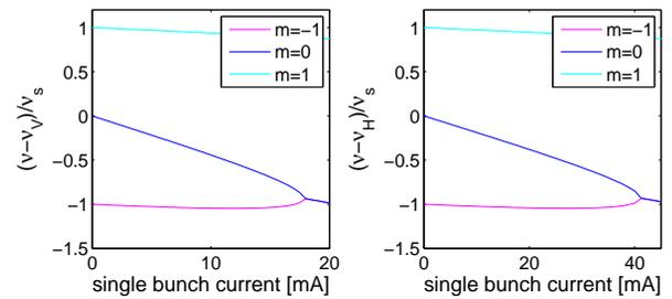
Figure 4: single bunch coherent mode detuning in phase I computed by MOSES, left vertical, right horizontal. The quadrupolar wake field is not taken into account.
