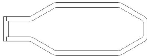
Figure 1: standard vacuum chamber made of stainless steel with its extension for connection with the antechamber
