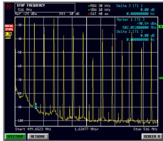
Figure 8: beam spectrum at 120mA shows a bump at higher revolution harmonics what is interpreted as a sign for the presence of ions
