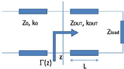
Figure 3: Transmission line model.
