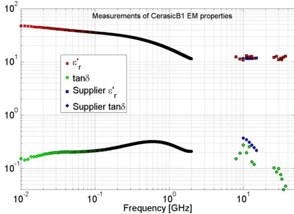
Figure 6: Measurements of real permittivity and loss tangent for SiC CerasicB1.
