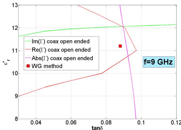
Figure 8: Contour plot for SiC EkasicF at 9 GHz.
