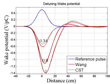
Figure 4: CST – Wang model [7] transverse quadrupolar wake potential comparison for SPS kicker MKE.61651 for  $\beta$  values 0.34, 0.8 and 1.
