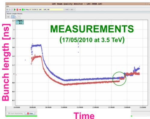
Figure 3: Bunch length increase during the instability.
