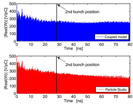
Figure 1: Time behaviour of the long range longitudinal wakefield for fundamental mode plus HOMs computed by fitting dispersion curve method (blue line) and Particle Studio (red line). The critical wakefield corresponding to the nominal 1% of charge fluctuation is equivalent to 1590V/pC.
