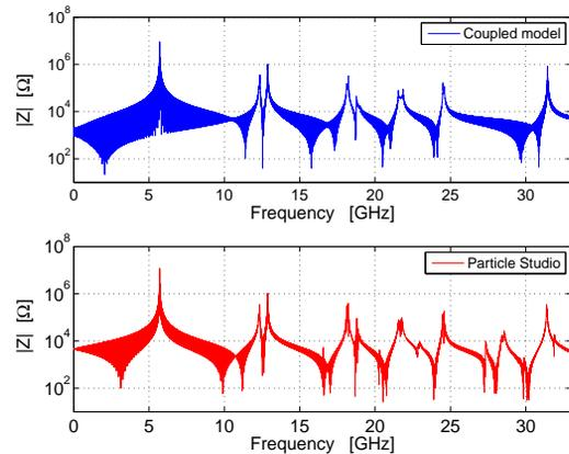
Figure 2: Impedance spectrum of the long range longitudinal wakefield produced by fundamental mode plus HOMs.
