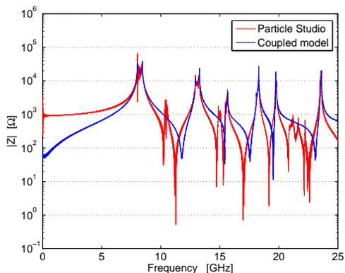
Figure 5: Impedance spectrum of the long range transverse wakefields
