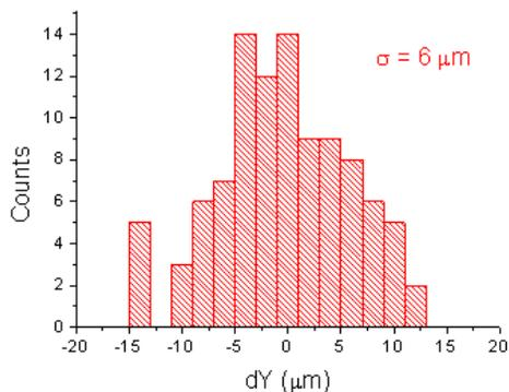
Figure 6: Relative position of the trailing bunch under the effect of a 5 V/pC/mm transverse wakefields
