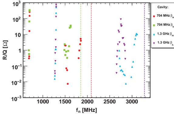
Figure 2:  $(R/Q)_{max}$  of the first three monopole bands. The dashed lines indicate the beam pipe cut-off frequency.
