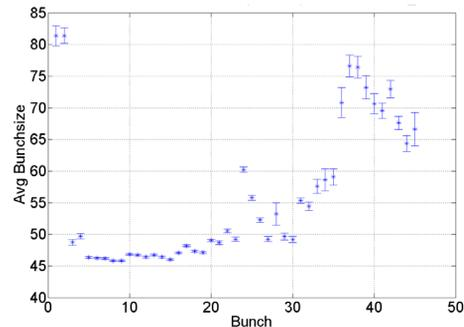
Figure 3: Vertical beam size measurements for a 45-bunch positron train at 4.0 GeV. The horizontal axis is bunch number and the vertical axis is the average vertical beam size. Large error bars indicate that the bunch shape is varying from one turn to the next.
