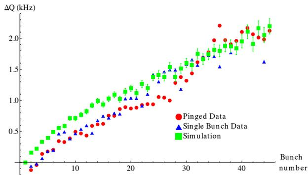
Figure 1: Vertical tune shift due to the electron cloud for all 45 positron bunches in a train at 4.0 GeV. The horizontal axis is the bunch number and the vertical axis is the tune shift with respect to the first bunch. The red dots are from pinged excitation, the blue triangles are single-bunch excitation data and the green squares are from a CESRTA electron cloud simulation[6].
