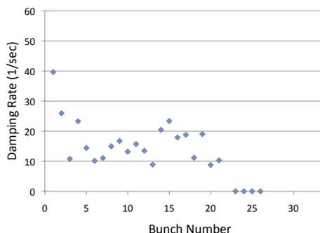
Figure 5: Damping rate of the vertical upper head-tail mode vs. the bunch number.
