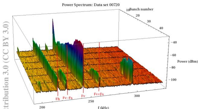
Figure 2: Self-excited beam position spectra for all 45 positron bunches in a train at 4.0 GeV. The horizontal axis is the frequency, the vertical axis is the spectral power and the third axis is the bunch number. (Bunch 45 is in the foreground.) Red lines locate the  $m = \pm 1$  vertical head-tail lines, and the horizontal and vertical tunes.
