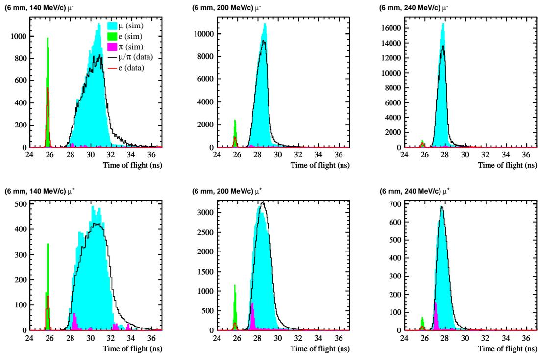
Figure 3: Time-of-flight between TOF0 and TOF1. Data vs Monte Carlo simulation for different 6 mm rad beams, at different energies.
