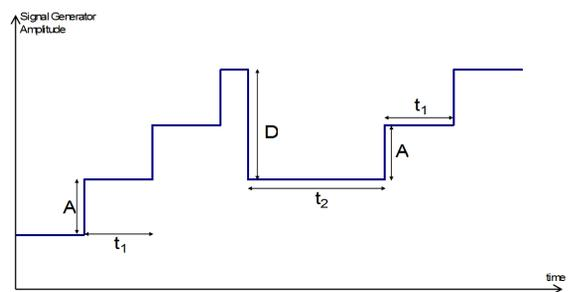
Figure 5: Graph showing how the ACS might vary the signal generator amplitude as a function of time.  $A$  is the fixed increment of the amplitude and  $t_1$  is the time between amplitude increments.  $D$  is the amplitude decrement and  $t_2$  is the time interval before the next increment, both of which are determined by the breakdown condition that was exceeded.
