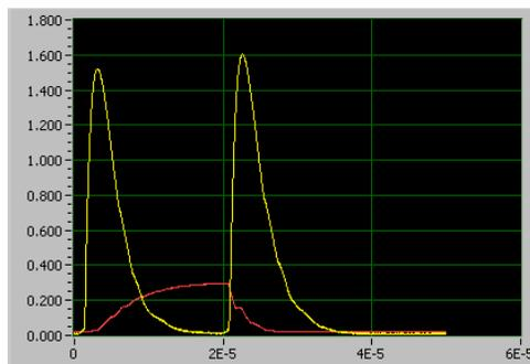
Figure 3: Reflected power (yellow) and pickup probe (red) signal after the envelope filter has been applied.
