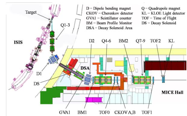
Figure 2: A schematic of the MICE beam line showing the magnetic lattice and detectors. The distance between GVA1 and TOF0 is approximately 6 meters. The proton absorbers are located just after D1 and before DS.
