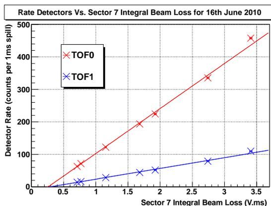
Figure 5: Scaler hits as a function of induced beam loss for the positive muon beam study (16th June 2010). Previously published in [3] (©2011 IEEE).
