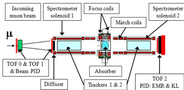
Figure 1: Step IV configuration of the MICE Experiment.
