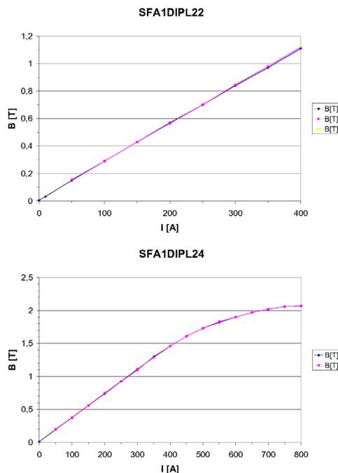
Figure 5: Plots of the  $B$ -fields of the chicane magnets as a function of current  $I$ .
