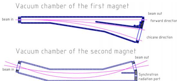
Figure 3: Technical drawing of the two chicane dipole chambers, with sketched in beam trajectories at maximum and minimum target angles.
