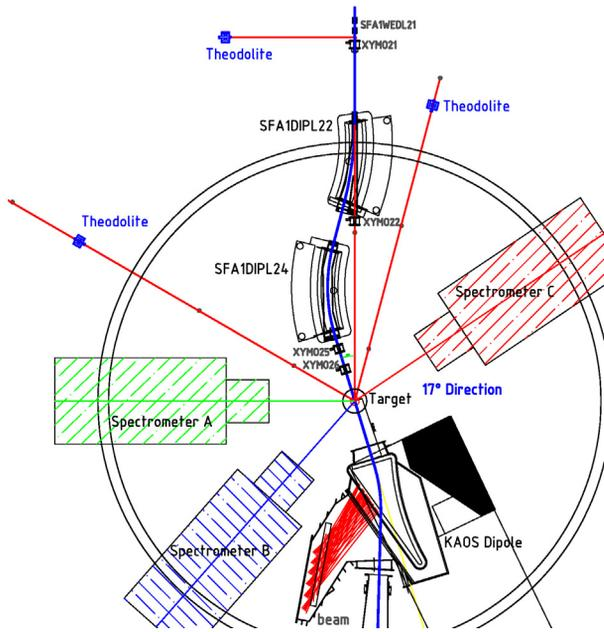
Figure 2: Overview over the KAOS chicane and the theodolite positions for target adjustment. The beam is coming from the top of the picture and is going to the bottom, following the blue line (17° target angle).
