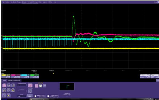
Figure 8: Scope display: first injection kicker (yellow), both extraction kickers (magenta and green) and the BPM signal from successive passes of the beam (cyan).
