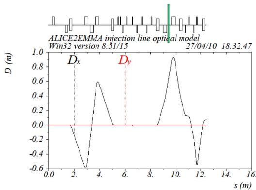
Figure 3: Dispersion in the EMMA injection line, with the YAG screen used highlighted in green.
