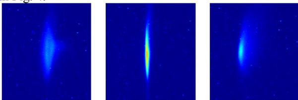
Figure 4: Variation of RF phase either side (left & right) of minimum energy spread (middle).
