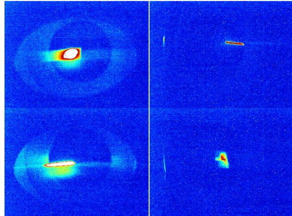
Figure 9: Extraction on the first YAG screen (L), the fourth (R); with RF (top), without RF (below).
