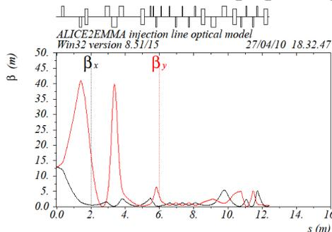
Figure 2: EMMA injection line layout and beta functions.
