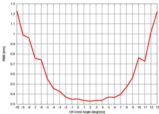
Figure 5: Beam size vs. off-crest angle.
