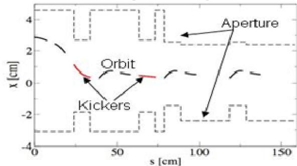
Figure 6: Injection region orbit, two normal cells (courtesy D. Kelliher).
