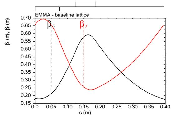
Figure 1: Beta functions for a single EMMA cell for the baseline model.
