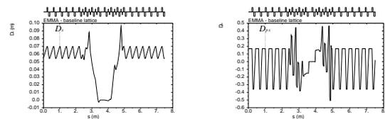
Figure 10: Dispersion and its derivative matched to zero in an EMMA straight.
