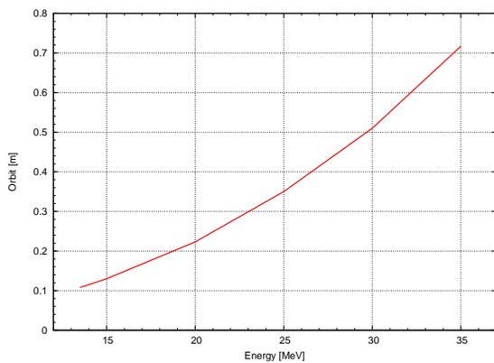
Figure 8: Orbit displacement vs. energy in the dispersion-free straight.
