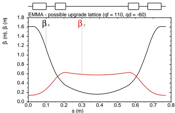
Figure 3: Beta functions when matching dispersion to zero in an EMMA straight at 15 MeV.
