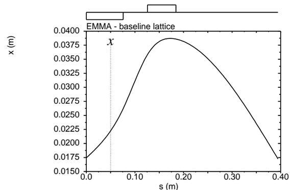
Figure 2: Orbit for a single EMMA cell for the baseline model.
