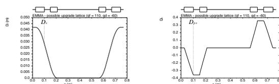
Figure 5: Dispersion and its derivative matched to zero in an EMMA straight at 15 MeV.
