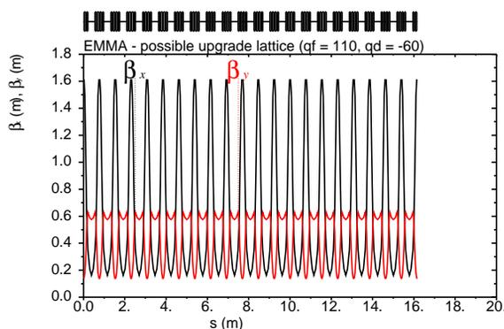
Figure 4: Beta functions when matching dispersion to zero in the EMMA ring at 15 MeV.
