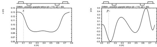
Figure 6: Orbit and angle when matching dispersion to zero in an EMMA straight at 15 MeV.
