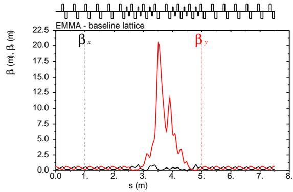
Figure 9: Beta functions with sextupoles used to match dispersion to zero in an EMMA straight.
