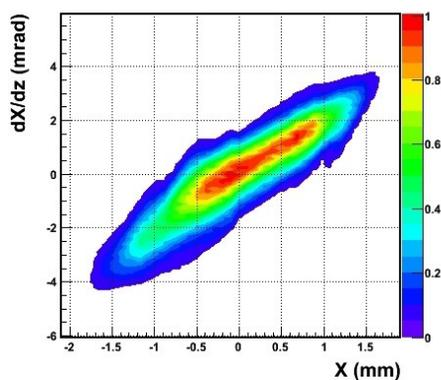
Figure 4: Horizontal phase space distribution of the 1 ns beam after the chopper.
