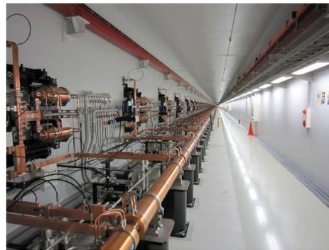
Figure 5: C-band acceleration system in the tunnel.
