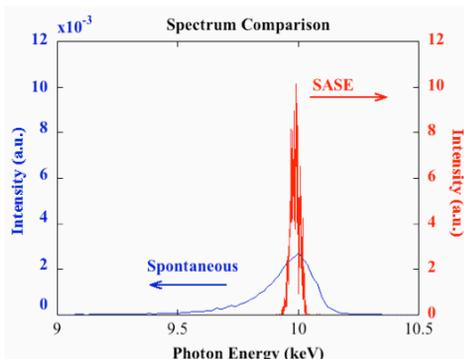
Figure 8: SASE laser spectrum at 10 keV.
