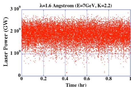
Figure 9: Laser power stability over 1 hr.
