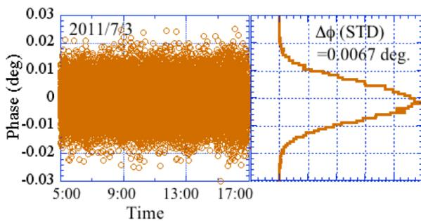
Figure 6: SHB phase stability over 12 hrs. Each data point represents an average of 10 shots.
