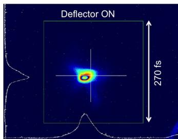
Figure 7: Vertically streaked profile of the fully compressed bunch.
