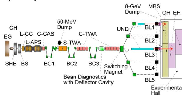
Figure 2: Schematic configuration of SACLA. EG, 500-kV electron gun; CH, chopper with collimator; SHB, 238-MHz sub-harmonic-buncher; BS, 476-MHz booster; L-APS, L-band alternating periodic structure (APS) typed standing-wave cavity; S(C)-TWA, S(C)-band travelling-wave acceleration tube; BC: bunch compressor; UND, undulator; BL, beam line; MBS, main beam shutter; OH, optical hatch; EH, experimental hatch.
