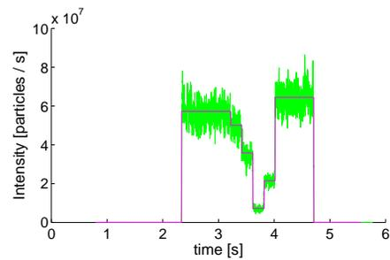
Figure 5: Spill with closed feedback-loop (green) and alternating reference-value (magenta).
