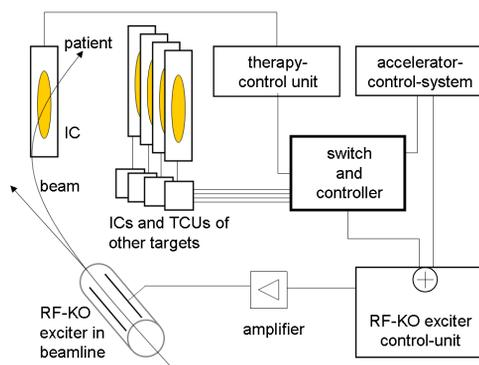
Figure 7: Set-up of feedback loop.
