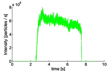
Figure 2: Typical spill achieved by RF-KO extraction. Here:  $E = 423 \text{ MeV/u}$ . Resolution:  $200 \mu\text{s}$
