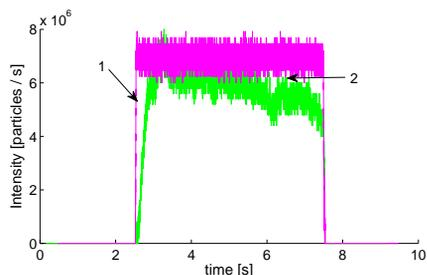
Figure 4: Comparison of spills with (magenta) and without (green) closed feedback-loop.
