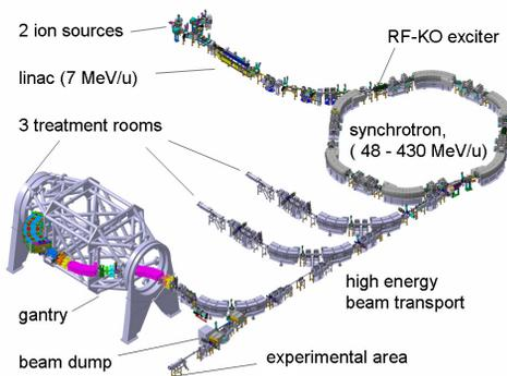
Figure 1: HIT accelerator complex.
