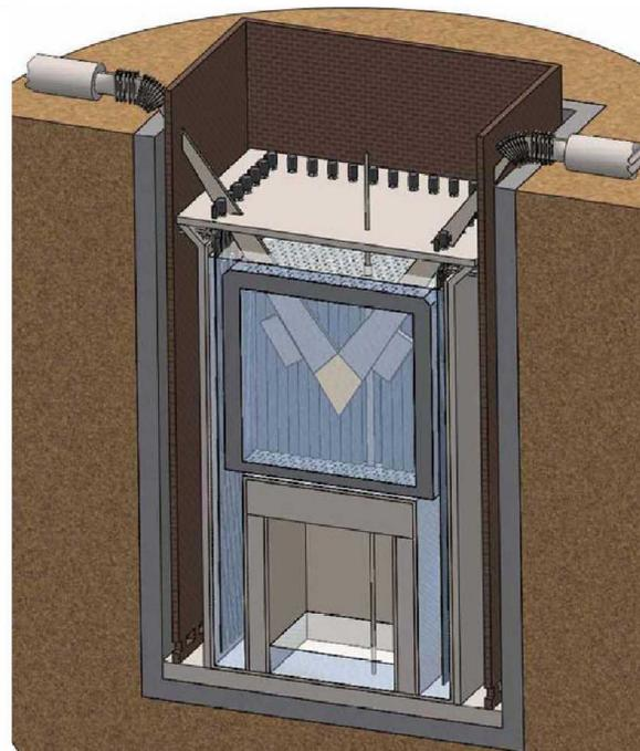
Figure 2: Conceptual design of the ADNA Green Energy Multiplier - Subcritical-technology, Thermal-spectrum, Accelerator-driven, Recycling molten salt reactor (GEM\*STAR) in its underground placement. The vertical dimension is about 9 m. The gray box is the graphite reflector for the core. Here, horizontal beams from two accelerators are shown at the top being bent by magnets into the core where they strike a uranium metal target shown schematically in the center of the core.
