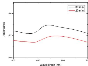
Figure 3: UV/VIS spectra of Au nano-particles producing by proton beam irradiation.
