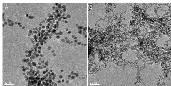
Figure 2: Surfactant controlled the shape of platinum nanoparticles. A. CTAB. B. Sodium dodecyl sulphate (SDS).
