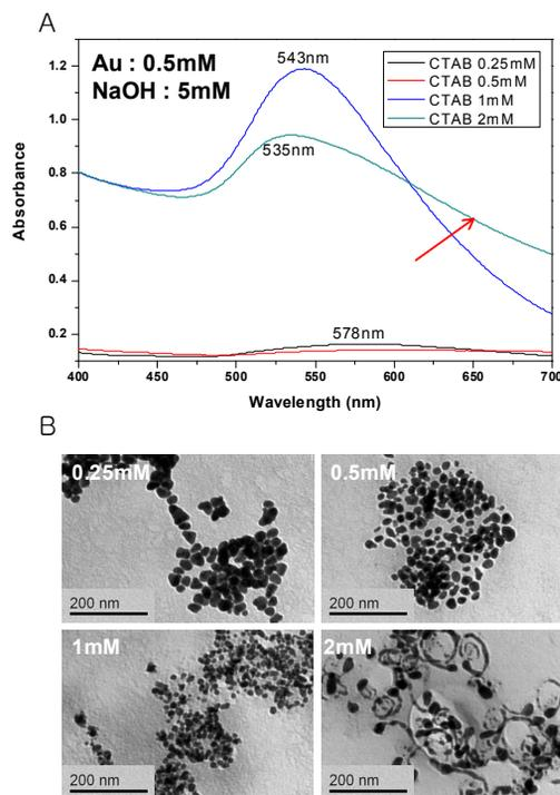
Figure 4: UV/VIS spectra and TEM images of difference conditions of NaOH and CTAB concentration. A. UV/VIS spectrum. B. TEM image.
