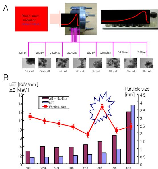
Figure 1: LET and energy effects of platinum nano-particle synthesis using proton beam. A. Slice sample stack and resulting proton beam irradiation. B. Particle size of various irradiation conditions.
