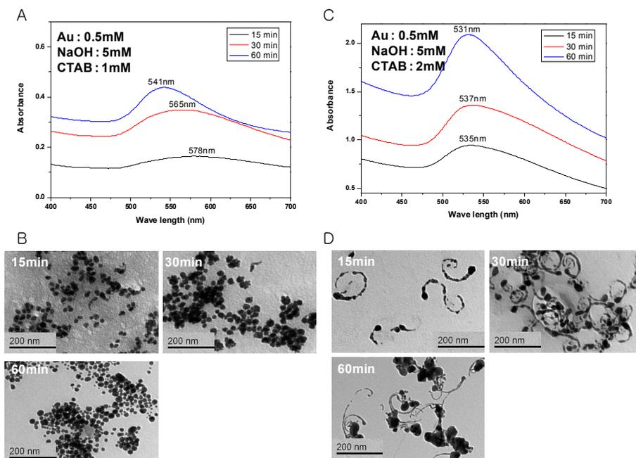
Figure 5: UV/VIS spectra and TEM images of effect of irradiation time of the proton beam on the formation of gold nanomaterials. A. UV/VIS spectrum of 1mM concentration of CTAB, B. TEM image of Figure 5A, C. UV/VIS spectrum of 2mM concentration of CTAB, D. TEM images of Figure 5C.
