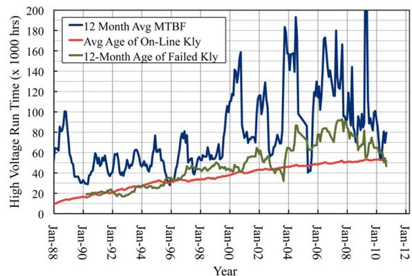
Figure 1: Run time statistics for the SLAC 5045 klystron.
