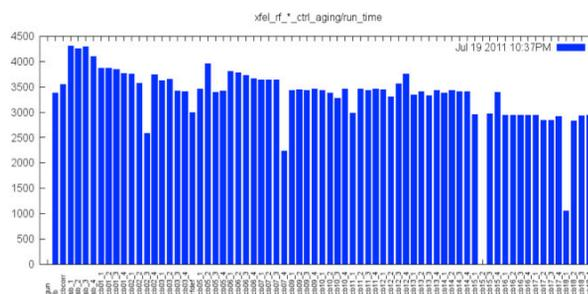
Figure 3: Run time hours for Toshiba E37202 klystrons. CB15-2 had a damaged pulse transformer and is not in use. CB18-1 failed after 1179 hours of operation.
