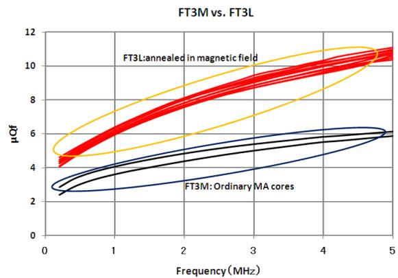
Figure 2: Characteristics of MA cores.  $\mu Qf$  is a product of permeability, Q-value and frequency and given by dividing the shunt impedance with a form factor. Red lines mean the characteristics of 8 different FT3L cores. Black lines mean maximum and minimum characteristics of FT3M cores in 2010.
