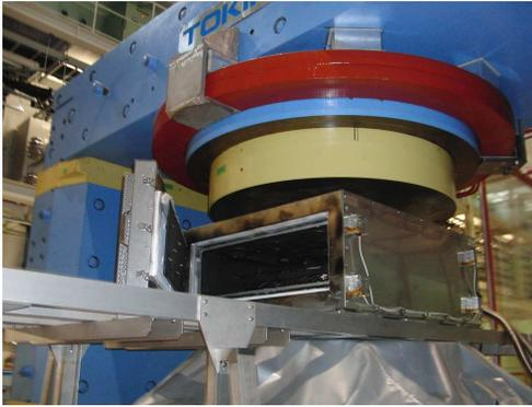
Figure 1: A large MA core production system using a cyclotron magnet. In a large magnet aperture, an oven is located.
