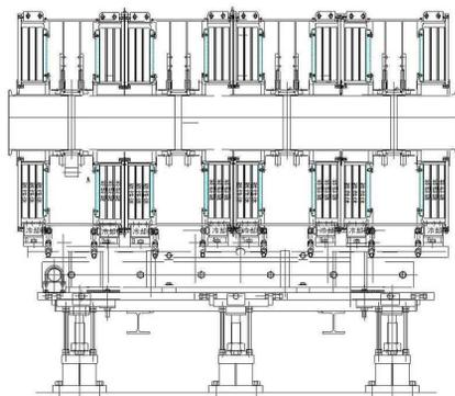
Figure 5: 4-Cell RF cavity for J-PARC upgrade.
