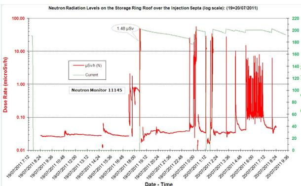
Figure 9: Neutron radiation levels above the injection point including a top-up test.
