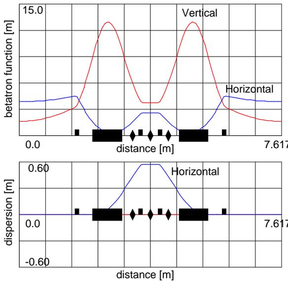
Figure 2: Lattice functions of ASTRID2.
