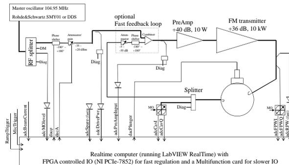
Figure 7: Block diagram of the new ASTRID LLRF.
