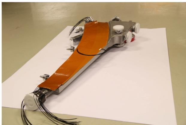
Figure 6: Picture of the pole-face winding placed on the dipole chamber, before fixation with kapton tape, and wrapping with insulation and aluminum foil.
