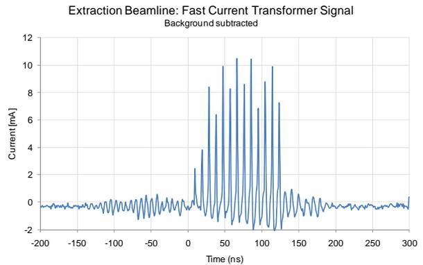
Figure 4: Signal from first fast current transformer in the transfer beam line.
