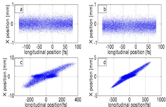
Figure 6: Simulation of the transfer of the femtosecond slice on SOLEIL ring. a) At the entrance of modulator. b) At the exit of modulator. c) At the exit of the radiator before CRISTAL beam line. d) At the exit of the radiator before TEMPO beam line.
