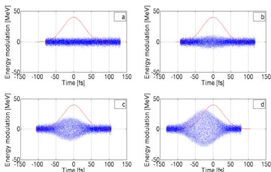
Figure 1: Simulation of the generation of the femto slice. a) Laser pulse at the entrance of modulator. b) Laser pulse at 1/4 length of modulator. c) Laser pulse in the middle of modulator. d) laser pulse at the exit of modulator. The time is the relative distance of the modulated electrons to the centre of the laser pulse.
