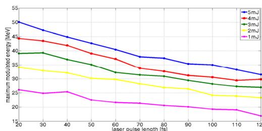
Figure 3: Maximum modulated beam energy versus laser pulse length under different laser pulse energy. The parameters used in the simulation are shown in Table 1
