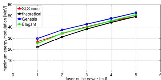
Figure 5: Comparison between the simulation results using SLS code, GENESIS, ELEGANT, and analytical formulae given in Eq.(4).
