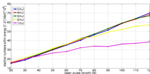
Figure 4: Number of electrons with modulated energy between 7 and 21 MeV versus laser pulse length under different laser pulse energy. The parameters used in the simulation are shown in Table 1.
