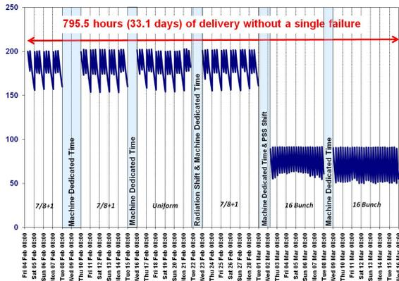
Figure 2: ESRF record delivery without a failure.
