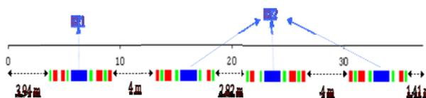
Figure 2: Arrangement of magnets in half a super-period of ILSF-Lattice-1. The blue arrows show the locations of dipole magnets.
