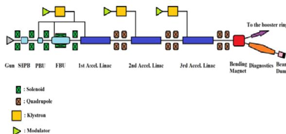
Figure4. Lattice layout of the pre-injector at ILSF.
