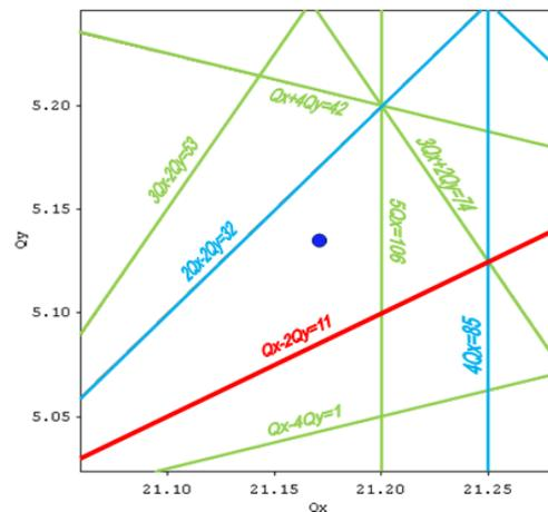
Figure 7: Tune point for the storage ring (2<sup>nd</sup> candidate).
