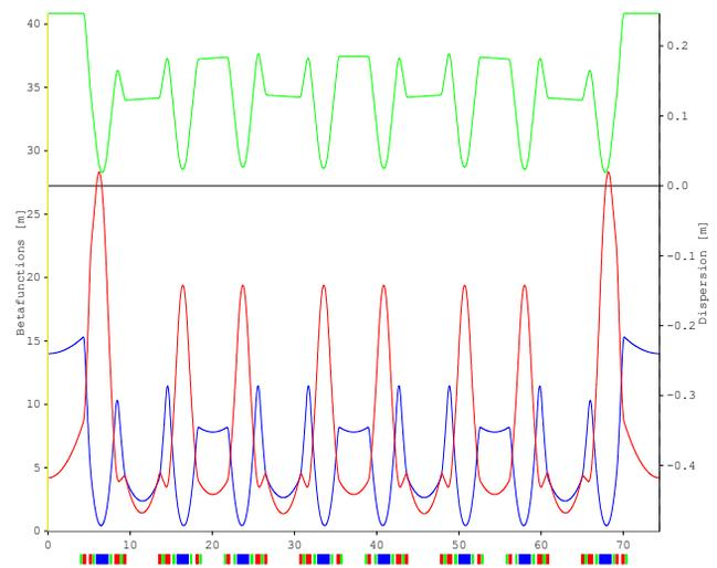
Figure 3: Optical functions in a quadrant of the ILSF storage ring (1<sup>st</sup> design). Blue and red curves represent horizontal and vertical beta functions respectively and the green curve remarks dispersion function.
