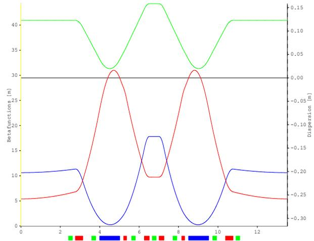
Figure 6: Optical functions in a super-period of the ILSF storage ring (2<sup>nd</sup> design). Blue and red curves represent horizontal and vertical beta functions respectively and the green curve remarks dispersion function.
