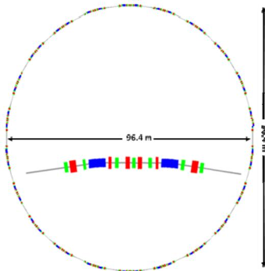
Figure 5: Layout of the ILSF storage ring (2<sup>nd</sup> candidate).
