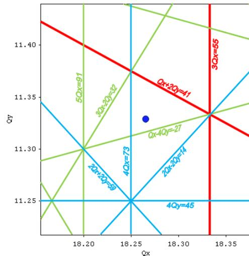
Figure 4: Tune point of the ILSF storage ring. The blue circle represents the tune point in tune diagram with 5<sup>th</sup> order of resonance line.
