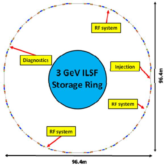
Figure 2: Layout of the ILSF storage ring (1<sup>st</sup> candidate).
