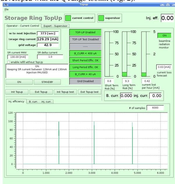
Figure 1: Top-up supervisor panel. The graph in the panel shows the injection events and the % of efficiency.
