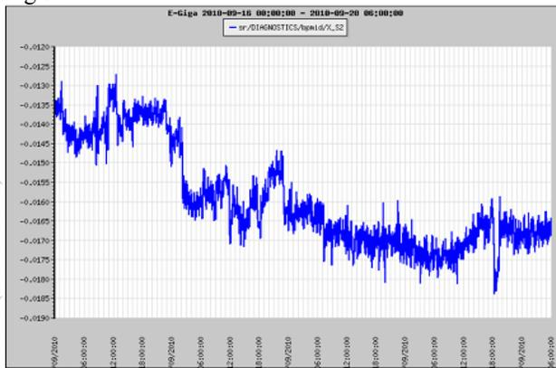
Figure 4: Horizontal orbit stability (y axis in mm) during top up for a period of 100 hours.
