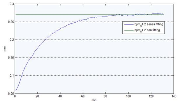
Figure 5: Bpm offset value drift towards “golden orbit” setting versus time after refill.
