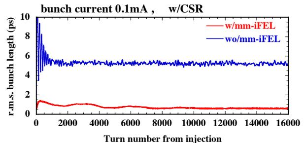
Figure 2: Turn-by-turn bunch lengths after the injection. Red and blue lines show those with and without the mm-iFEL accumulating the peak power of 1.8 GW, respectively.
