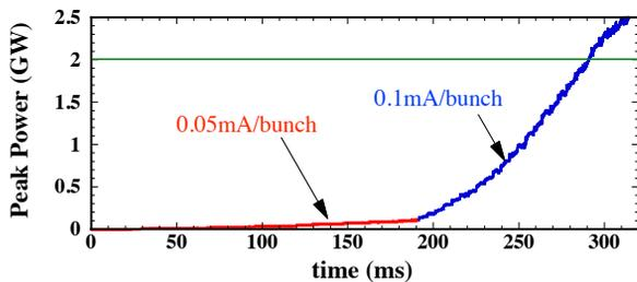
Figure 4: Simulated peak power growth in the MWR by drive bunches with bunch length of about 3 ps (r.m.s.). Red and blue lines show the power growth from zero to 0.11 GW by the drive beam with 0.05 mA/bunch and from 0.11 GW to 2.0 GW by those of 0.1 mA/bunch, respectively. The drive bunch numbers are increased one-by-one every 4.79 ms corresponding to 1000 turns.
