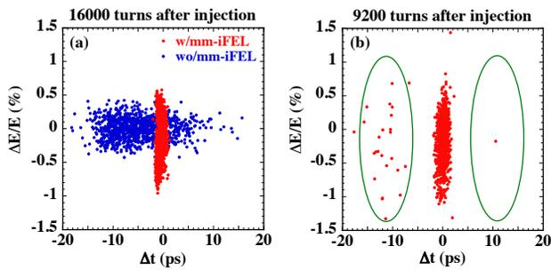
Figure 3: (a) Longitudinal phase space distributions at the 16000 turns after the injection. Red and blue dots show those with and without the mm-iFEL when the peak power is 1.8 GW. (b) The phase space distribution with the mm-iFEL when the peak power is 1.6 GW. The electrons in the green circles are spilt out of the middle specified mm-wave bucket.
