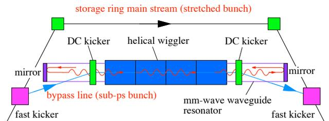
Figure 5: A possible layout of the mm-iFEL system placed on a bypass line assumed to be inside the storage ring and parallel to the long straight section.
