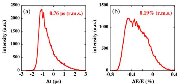
Figure 1: (a) Temporal and (b) momentum bunch profiles at an injection point of the storage ring after passing through the designed XFEL-to-Storage Ring transport line. The calculations include the CSR effect when a bunch charge is 479 pC.
